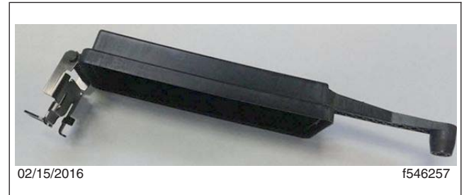
Fig. 6, Hinge Bracket Installed on the Cover
