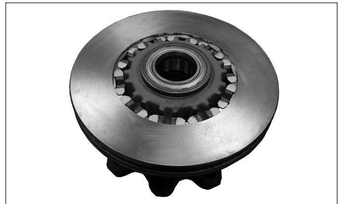
Figure 90 – Intermediate Elements (Spacers Installed)
