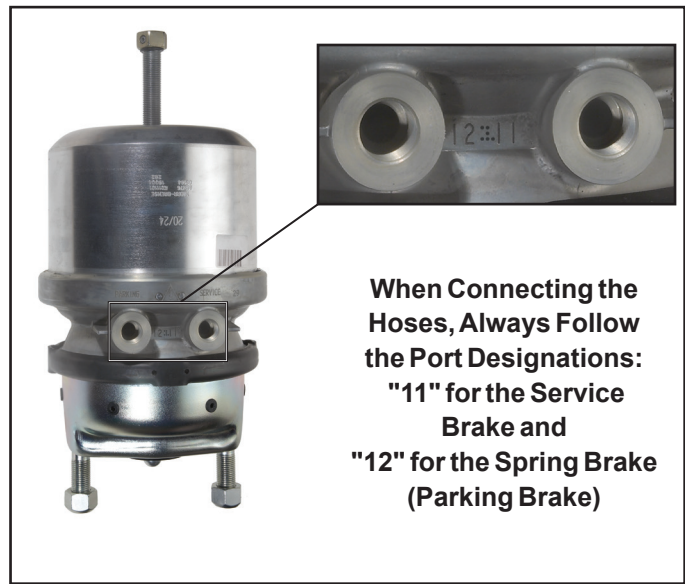
Figure 12 – Bendix® Piston-Style Spring Brake Port Connections
